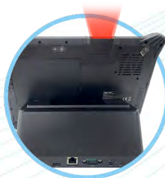
2D Scanner & Comprehensive Charging Dock*
